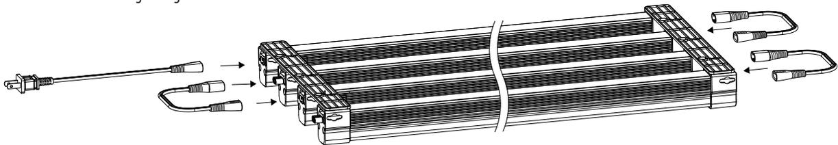
**5** Install the hanging cables on to the 12 in. brackets. Then attach the other end of the hanging cables to the hanging hooks (not provided) mounted on ceiling.
