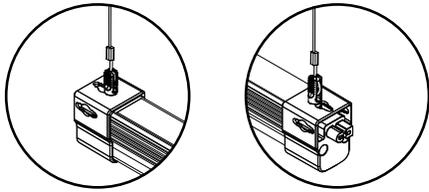
**5** Hang the hanging cables onto the hanging hooks.
