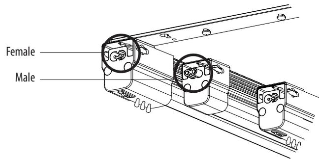
**4** Install the 5 ft. power cord into the outlet of the first grow light's end cap. Use 6 in. linkable cables to connect all grow lights.
