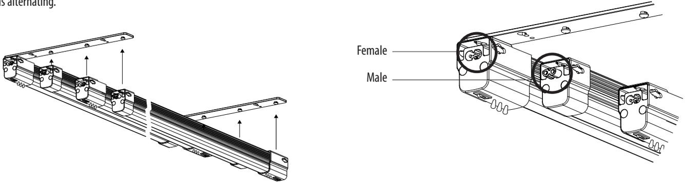
**3** Use the above assembly as a template. Place against the ceiling and mark mounting holes.
