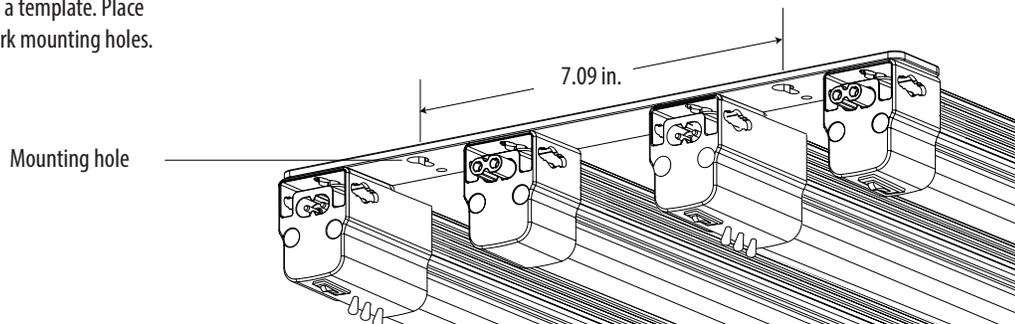
**4** At the marked locations, drill holes for the screw or anchor as appropriate.
