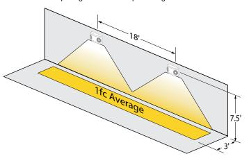
Using multiple LEM54-N4 units mounted at a typical 7.5' height delivers 12' on center spacing with a 6' wide path of egress.
