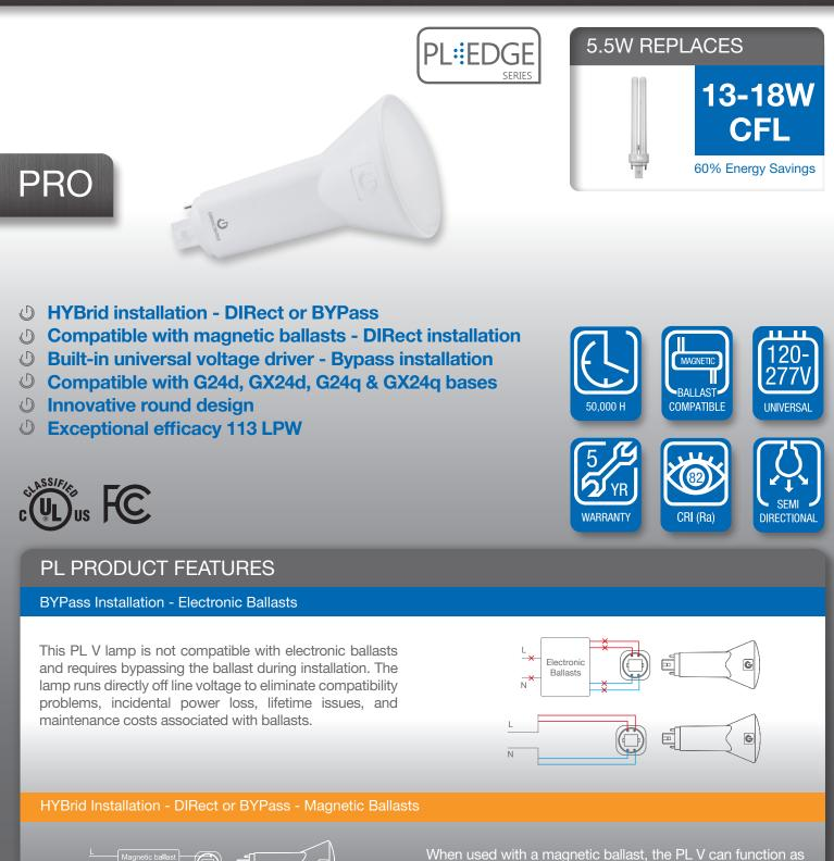
a plug & play lamp and operate with the existing ballast. If the ballast is not compatible, it can be bypassed and the lamp can run directly off line voltage.
